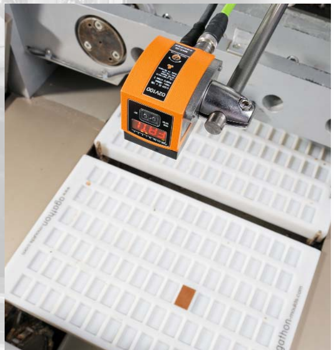
The vision sensor checks if the chocolate mould is empty before it is refilled.
