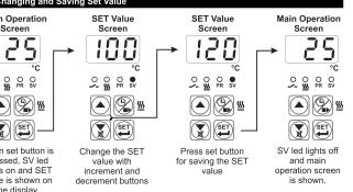
SET value changes according to maximum and minimum value of device type and scale. It can
