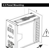
1-Before mounting the device in your panel, make sure that the cut-out is of the right size
