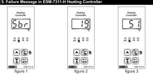
1- Probe failure in analog inputs. Sensor connection is wrong or there is no sensor connection When this message is on the screen, if buzzer function selection parameter  $\lceil b \rfloor \Gamma \rceil$  is 3 or 4, internal buzzer starts to operate. See figure 1.
