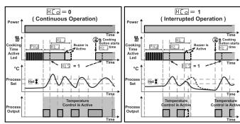
2-When cooking time parameter □ ≥ 1, if selection of temperature control and starting the cooking time parameter □□ = 1 (Temperature control starts at power on. Cooking time (Timer) can be started by pressing cooking ON/OFF button or when cooking time start/stop input is getting closed condition) is selected;
