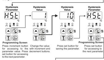
If no operation is performed in programming mode for 20 seconds, device turns to main operation screen automatically.
