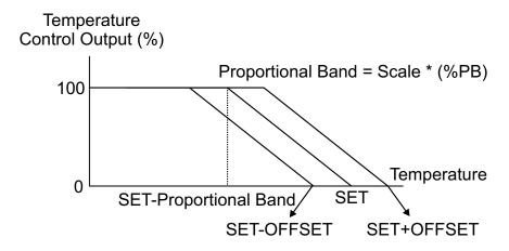
When temperature is not equal to SET value, to remove the difference between SET value and temperature and to make equal the temperature and SET value, set offset is used. It can be adjusted from -20% to 20% of full scale.
