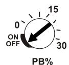
Trimpot is adjusted to point out ON/OFF part for ON/OFF Control form.
