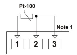
3-wire Pt-100 connection (with line compensation) (Max. Line impedance is 10  $\Omega$ )
