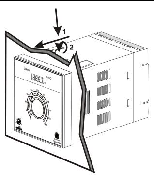
The unit is designed for panel mounting.
