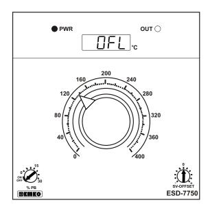
Sensor failure in analogue inputs.
