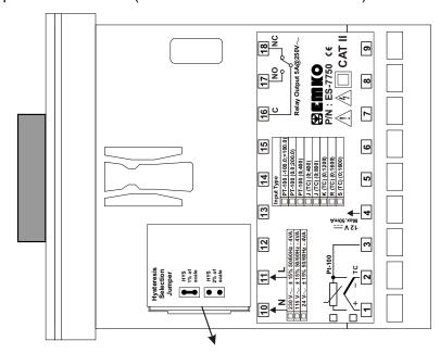
Jumper is under cover and cover is on top side of the device
