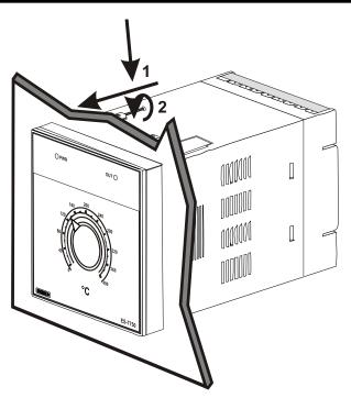
The unit is designed for panel mounting.
